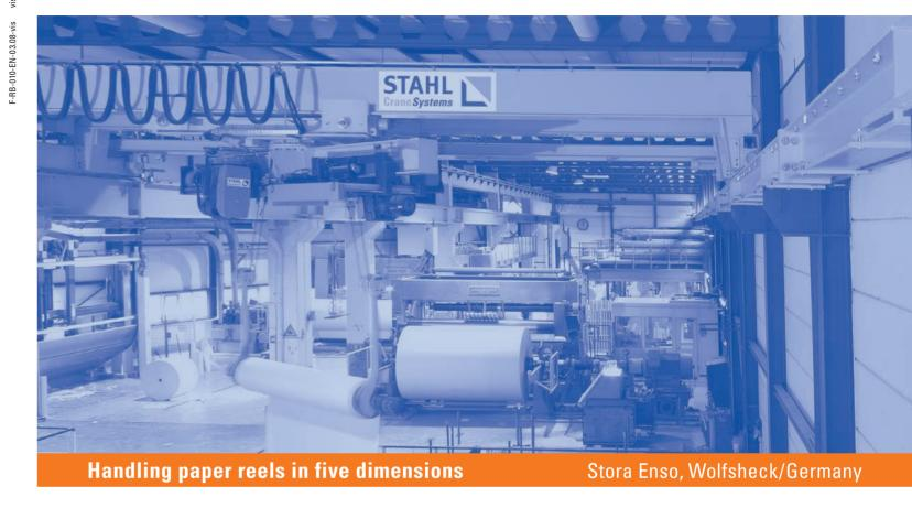
Crane type Double girder overhead travelling crane for handling paper reels \_ S.W.L. 2x9,000 kg \_ Span 11.0 m
