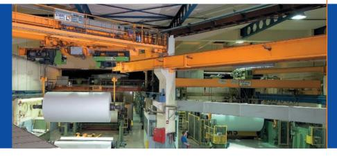
Handling reels of paper weighing several tonnes is one of the most demanding applications in crane technology. In paper factories, extremely heavy loads must be transported with millimetre precision. The cranes' capacity must be available right around the clock since production downtimes entail high costs. Only competent crane manufacturers with well-founded engineering know-how, reliable logistics and comprehensive service can meet these requirements.
