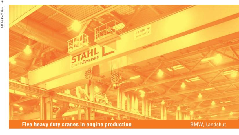
Crane types 5 ZL-A double girder overhead travelling cranes by STAHL CraneSystems \_ S.W.L.'s 4x40,000 kg and 16,000 kg \_ Spans 28.65 m/21.5 m/13.5 m \_ Drives Stepless speed control \_ Equipment S7 SPC control, condition monitoring package (SSC load cumulation, load monitoring at hook, SMC load spectrum memory, motor and brake management), electrically rotating hooks, temperature control of all motors, maintenance platform along crane bridge, radio remote control
