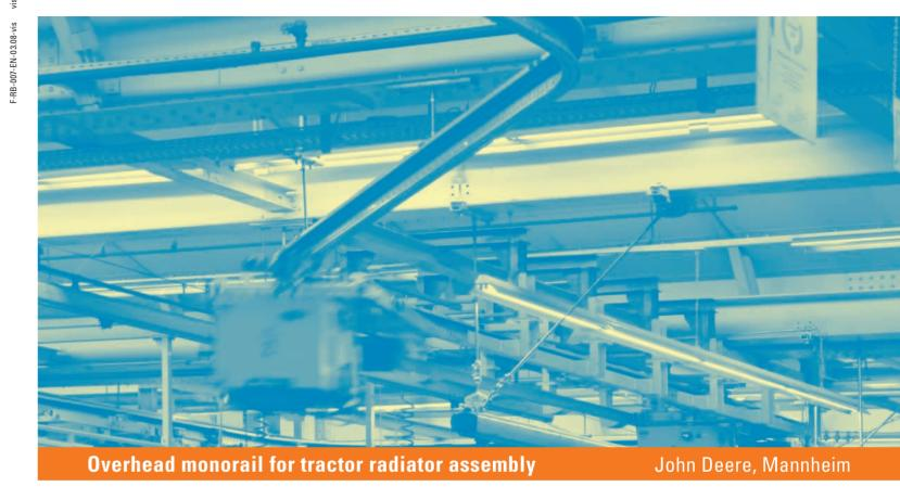
Type of installation circular runway in special KT2000 profile \_ Length of runway 93 m with maintenance spur Trolleys \_ 8 monorail trolleys, each 250 kg S.W.L. \_ Hoists STD 1005-8/2 2/2-2E dual chain hoists \_ Power supply eight-pole conductor line integrated into system \_ Equipment radio remote control with redundant infrared signal, travel speed synchronised with assembly line, chain hoist at right-angles to runway, can be moved on special skid
