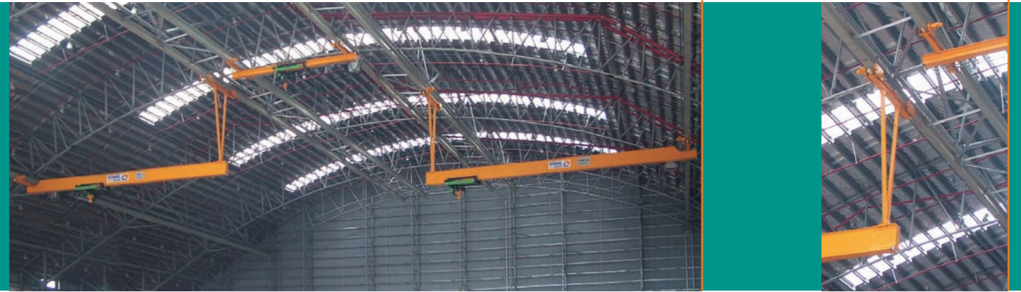
The central crane is mounted directly below the ceiling and operated on a separate crane runway. This ensures clear access for the aircraft.
