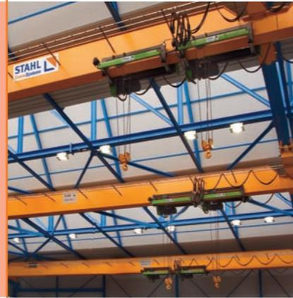
The offset crane girder design of STAHL CraneSystems enabled the maximum effective hook path to be achieved in spite of the very low ceiling. The additional suspended trolley in the centre made the span of 51 m possible.
