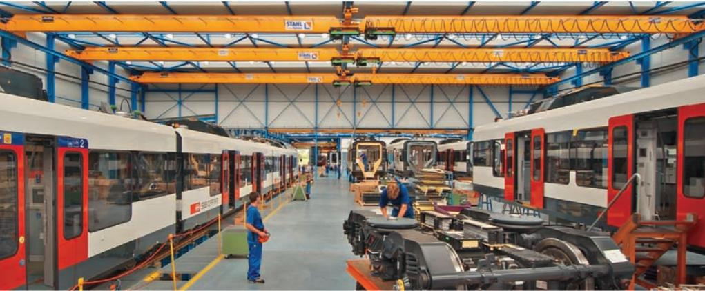
All three single girder hybrid cranes can combine in synchronous operation to transport loads up to 45 t.
